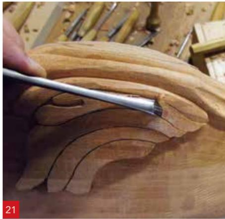
**22** For the very tips of the leaves use No.3, 8mm and No.5, 8mm carving gouges to round and clean up the edges
