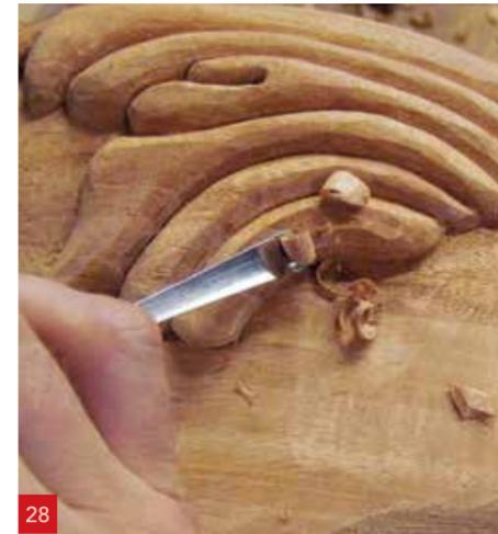
**28** On the very last leaf, carve a concave cove into the outer edge of the leaf using a No.5, 8mm carving gouge
