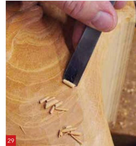
**29** Clean up all the carving gouge marks left on the leg itself. Use No.2, 14mm and No.2, 20mm carving gouges to shave the wood as flat and clean as possible
