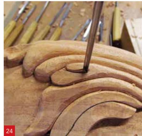
**“Repeat the stab and relief cuts to remove the waste wood”**
