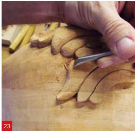
**24** To carve the detail into the eyes of the acanthus leaf, start by stab cutting the smaller inside radius with a No.8, 3mm carving gouge. Then, on the larger radius just above the eye, use a No.8, 7mm gouge and on the two straight sections use No.3, 12mm and No.5, 8mm carving gouges. Repeat the stab and relief cuts to remove the waste wood until you have reached around 6mm deep
