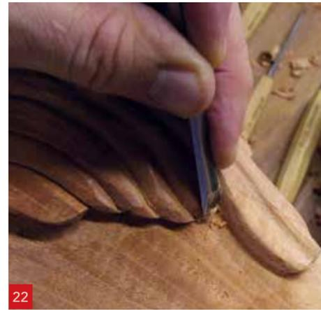
**23** On the upper part of the wing/leaf use a No.3, 12mm carving gouge upside down to radius the top closest to the centre. Then flip the gouge back over to carve the concave section of the wing
