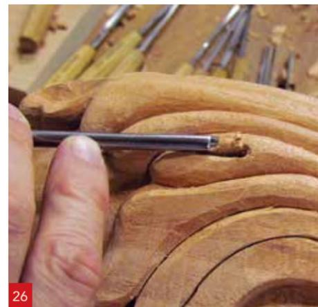
**27** On the outer ends separate the leaves from each other as you did in step 10 by using a No.3, 12mm carving gouge upside down and carving arches on the faces of the last two remaining leaves on both sides. Then with a No.5, 8mm carving gouge, radius and clean up the top and bottom ends of the leaves
