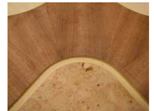
The finished plough ready for solid black ebony banding
