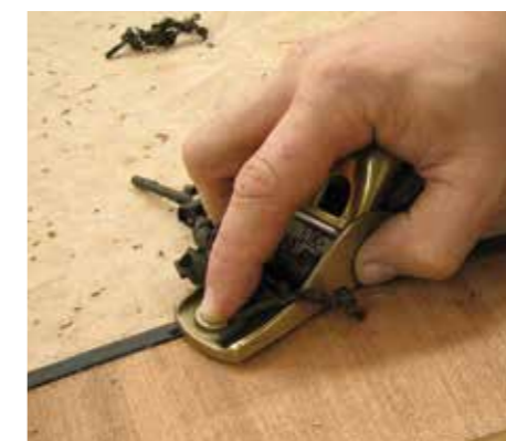
Remove the bulk of the banding with a block plane
