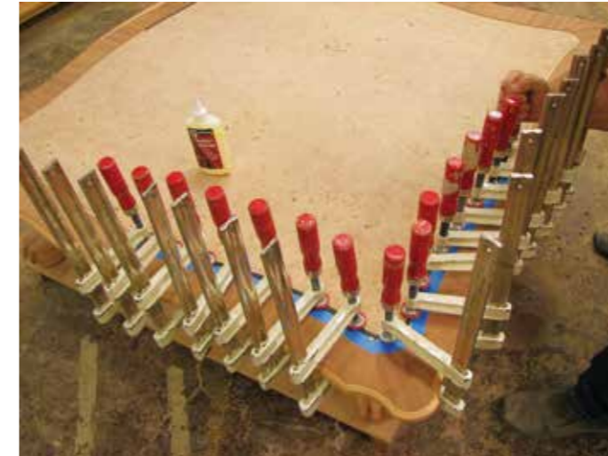
Glue and clamp the solid ebony banding into the corner of the top
