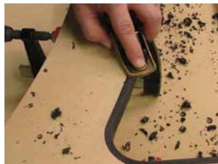
Hand plane the ebony inlay flush to the template
