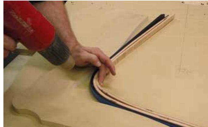
Use a heat gun before gluing the layers together
