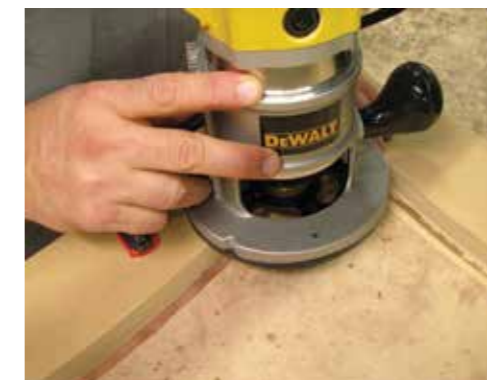
Rout in the plough by following the template edge with the bushing guide
