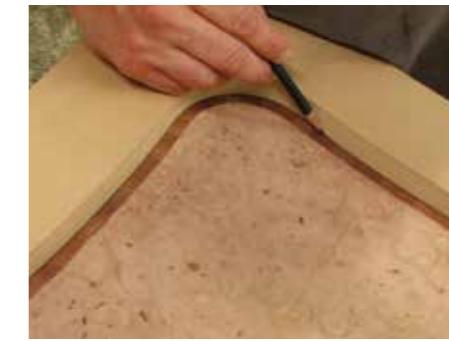
Draw in the pencil line around the entire top to ensure the same 10mm spacing, also blending the larger radiuses at the sides of the top
