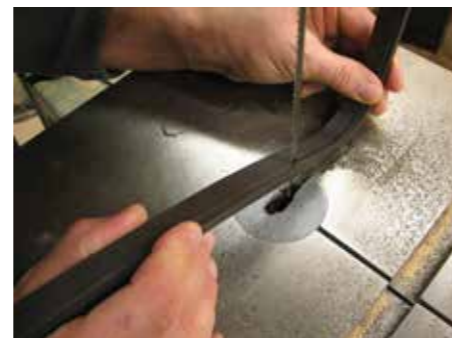
Use a bandsaw to cut out the ebony banding
