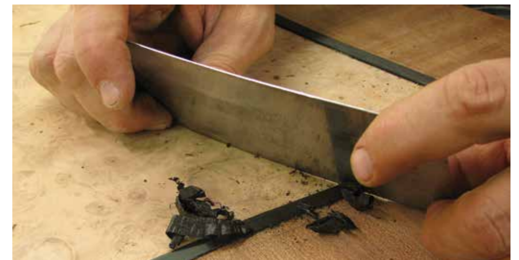
Use a cabinet scraper to take the ebony flat and smooth to the veneer
