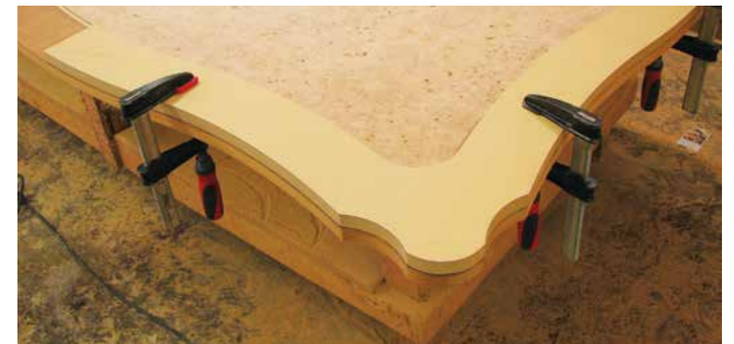
Clamp down template A using three small bar clamps
