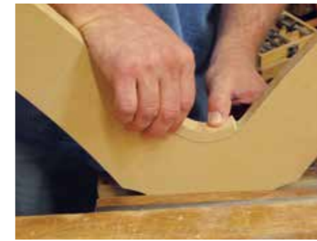
Sand the edges of templates A and B using sandpaper stuck to the falloff MDF made into sanding blocks
