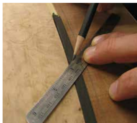
Mark out the mitre line on the top face of the banding
