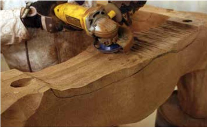
**22** Using the coarse grinding wheel to remove the bulk of the wood
