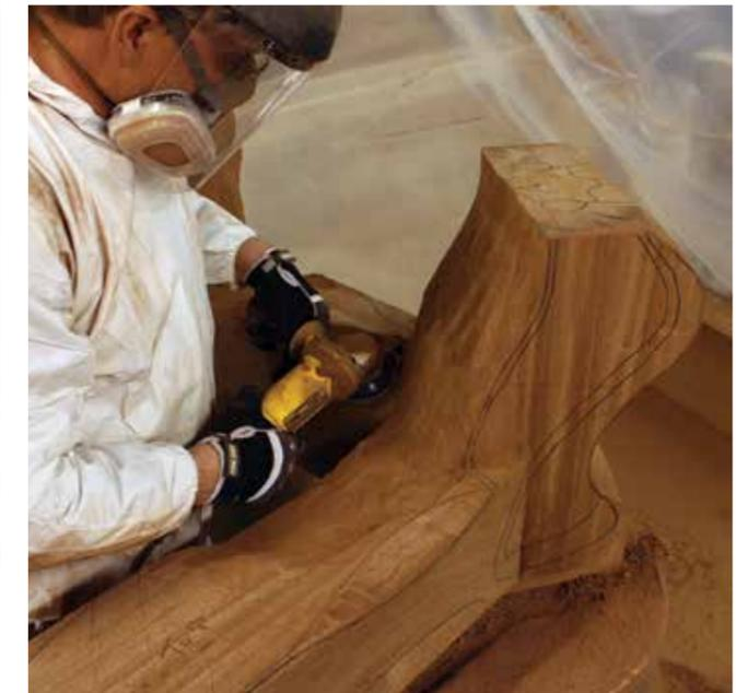
19 Grinding one leg at a time to remove the back side of the leg
