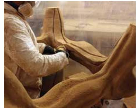
**26** Using the side of the grinding wheel to cut into the hardwood
