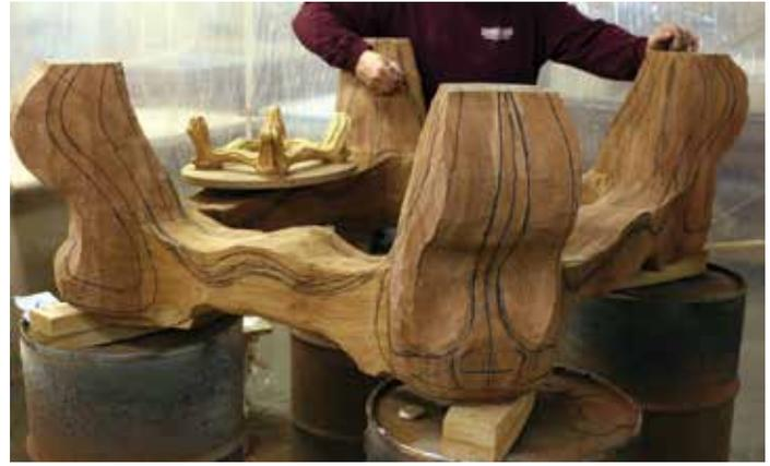
**23** Redrawing the lines back onto the base so they are closer to the true shape
