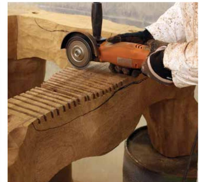
21 Adding depth cuts to the bottom of the runners
