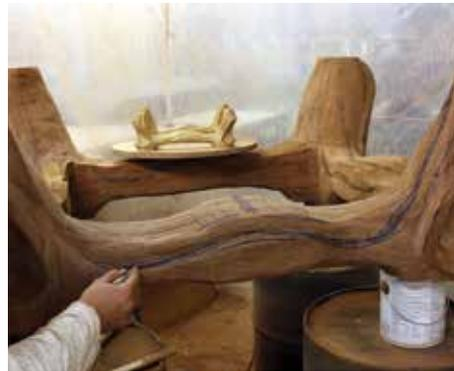
**25** Draw in the next set of lines to where the deeper cuts will blend with the legs and runners
