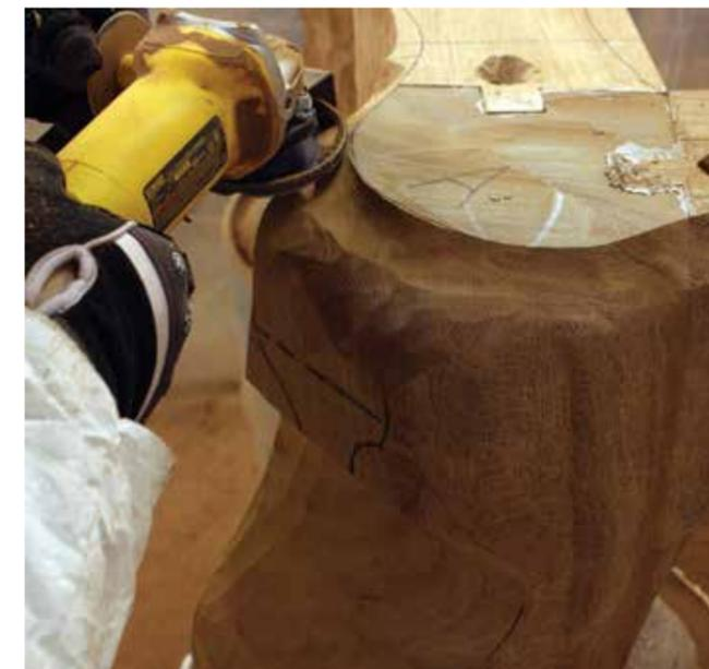
20 Grinding the bottom of the legs to reach the radius shape
