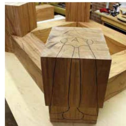
14 Using a marker pen to go over all the pencil lines drawn on the base system
