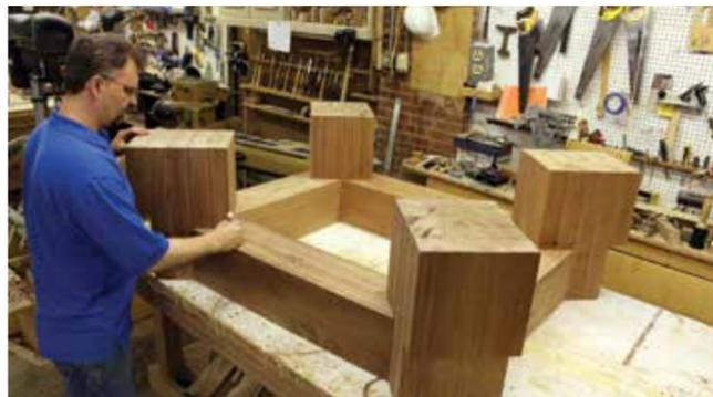
10 Laying out the base system to mark where each end and face will be located
