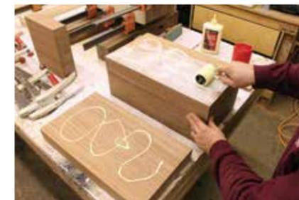
5 Rolling glue onto the surfaces
