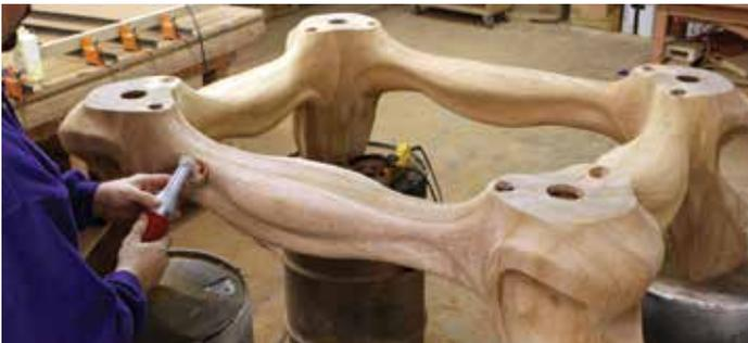
**27** Smoothing out the curves and twists using a smaller grinder with a medium 50mm diameter grinding wheel
