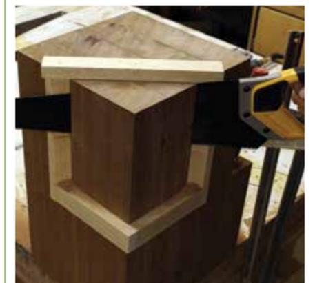
7 Cutting a 45° angle on both lower back sides of all four legs
