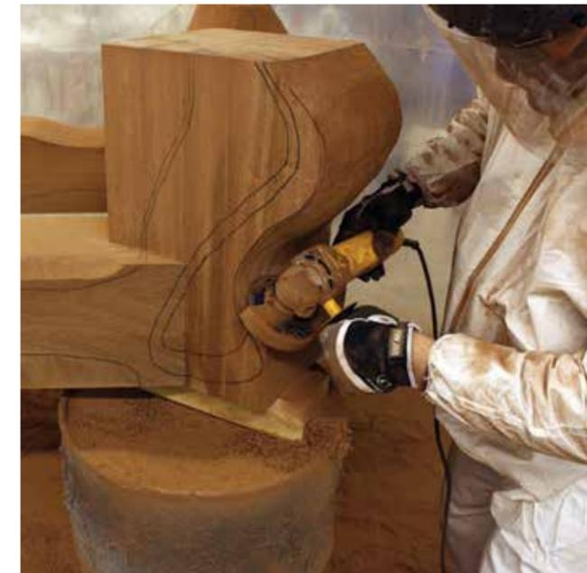
18 Using a grinding wheel with durable tungsten carbide with my hands in a safe position
