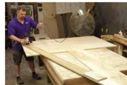
Routing out the large radius clamping jig
