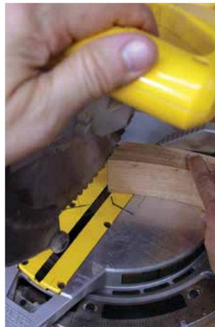
Cut the mitres with a mitre saw
