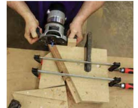
Routing the dovetail dado into the ends of the straight aprons
