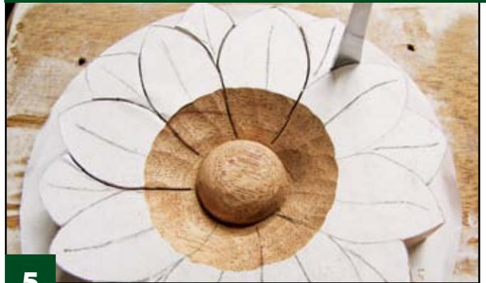
**5** **Make stop cuts around the petals.** Redraw the petal lines in the carved area around the center circle. Match the profile of the gouge with the curve of the petals; I use ½" (or 12mm) #2, #3, and #5 gouges. Tap the gouge with a mallet to make stop cuts about ⅛" (3mm) deep around each petal.
