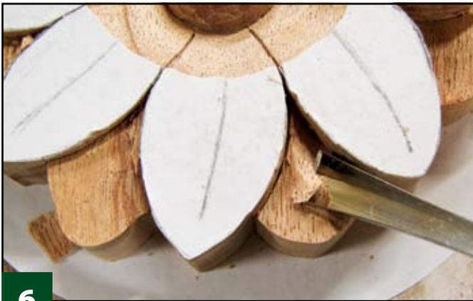
**6** **Carve the small petals.** Use the ½" (or 12mm) #3 fishtail gouge to relieve up to the stop cuts on all of the eight small outer petals. Repeat the process until the smaller petals are ½" (13mm) deep at the inner point and ⅜" (10mm) at the edge of the petal. Use a ⅛" (3mm) #3 gouge to carve the inner point.
