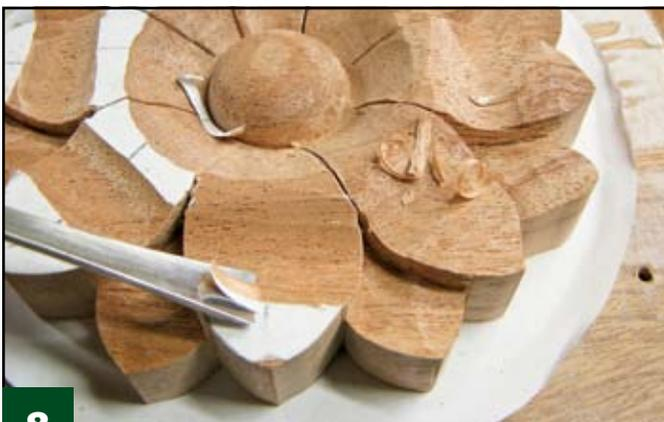
**8** **Refine the petals.** Use the ½" (or 12mm) #5 fishtail gouge to remove the sharp edges from the groove and blend the petal from the center to the outer tip. Shave off small amounts of wood and work your way around the flower to smooth all eight petals.
