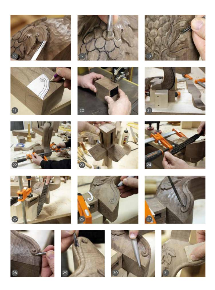
16 Next, I started carving the leaves by cutting a concave centre cut approximately ¼in deep with a No. 9/5 carving gouge. To give the leaves a realistic appearance I carved a gradual slope from the outside edges to the centre of the leaves. I used a few flatter gouges to shave off small amounts at a time until I achieved a smooth, natural flow on each grape leaf.
